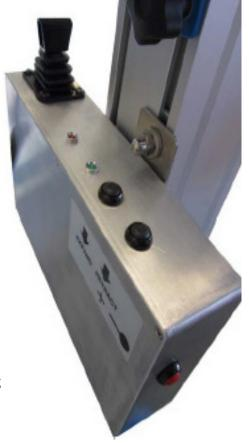
Always rotate the roll to a horizontal position and retract as soon as possible after lifting. Leaving the core expanded for more than a few minutes will result in a fault warning. See trouble shooting for a detailed description of this.
