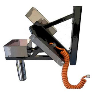
To prevent accidental unloading, the roll is freed by a two-hand grip. When the reel is gripped, it is rotated steplessly by a joystick or a crank handle and can be positioned vertically or horizontally. The expander is equipped with small rollers on the top side to aid the unloading of heavier reels.
